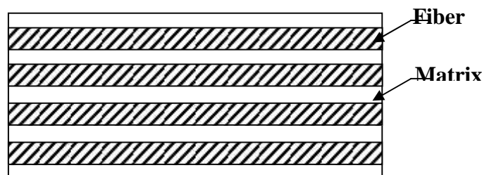
Fig. (1) Structure of a fibrous composite
